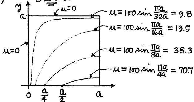
The sketch should be "topologically correct" — i.e., in its key features. In particular, each isotherm must be horizontal at the  $x=a$  edge because  $u_x(a,y)=0$ .
