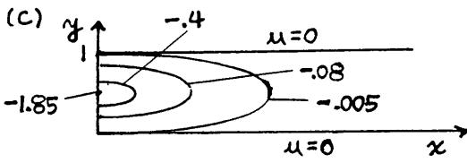
$u$  will be negative at each  $(x,y)$  in the interior of the domain. Its largest negative value will be at  $(0,0.5)$ , and the isotherm values will increase and approach zero as the isotherms penetrate more deeply into the strip.
