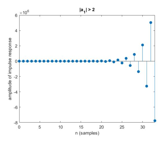
So accordign three different figures under different value of  $a_1$ , we can find only when  $a_1 < 2$ , the system has the stable impulse response. (i.e. both poles has to be located inside the unit circle, the system would be stable.)
