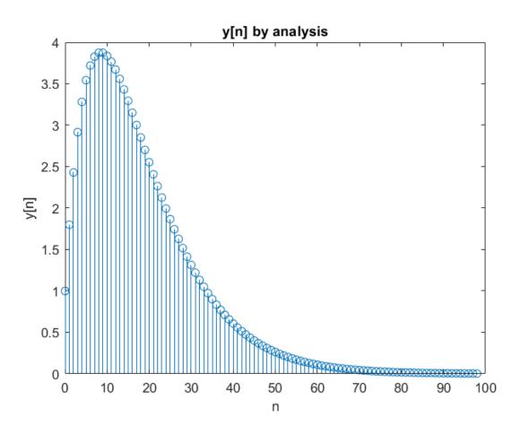
(b) Take first 50 samples of x[n] and h[n]. Compute and plot y[n] using the conv function.
