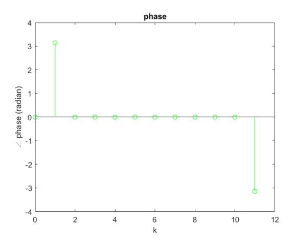
8. (8%) Consider a noncausal finite length sequence  $x[n] = \delta[n + 1] + \delta[n] + \delta[n - 1]$ , we can compute the DTFT in MATLAB using following scripts:
