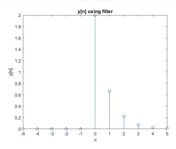
As shown in the output sequence y and its plot, y[n] is equal to  $2 \times \left(\frac{1}{3}\right)^n u[n]$
