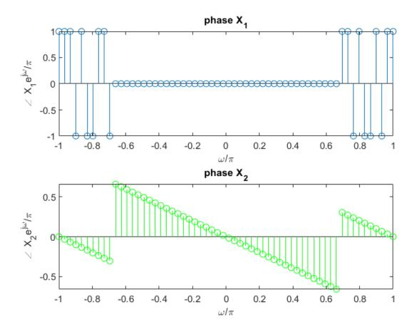
(b) Is the magnitude |X1|=|X2|? Is the phase  $\angle X1=\angle X2$ ? If not, Explain. Ans: the magnitude is the same, but the phase it different. Fourier transform is
