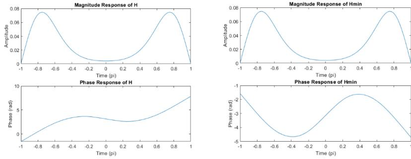
We can find that  $|H_{\min}(s)| = |H(s)|$  and  $\angle H_{\min}(s) < \angle H(s)$
