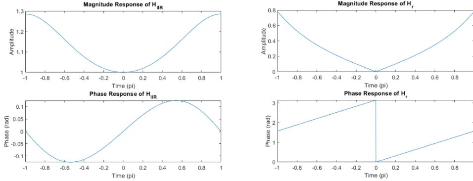
We can see the curve of magnitude response of  $H_{IIR}(e^{j\omega})$  is smoother and larger than magnitude response of  $H_r(e^{j\omega})$ .
