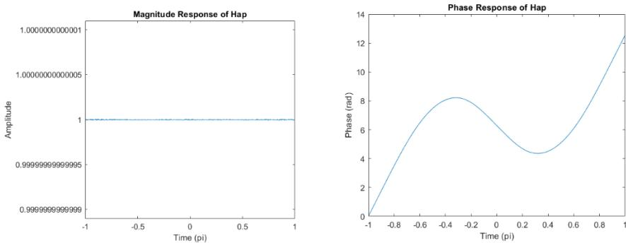
We can find that  $|H_{ap}(s)| = 1$  and  $\angle H_{ap}(s) + \angle H_{\min}(s) = \angle H(s)$
