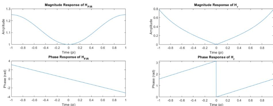
We can see the curve of magnitude response of  $H_{FIR}(e^{j\omega})$  is smoother and larger than magnitude response of  $H_r(e^{j\omega})$ .
