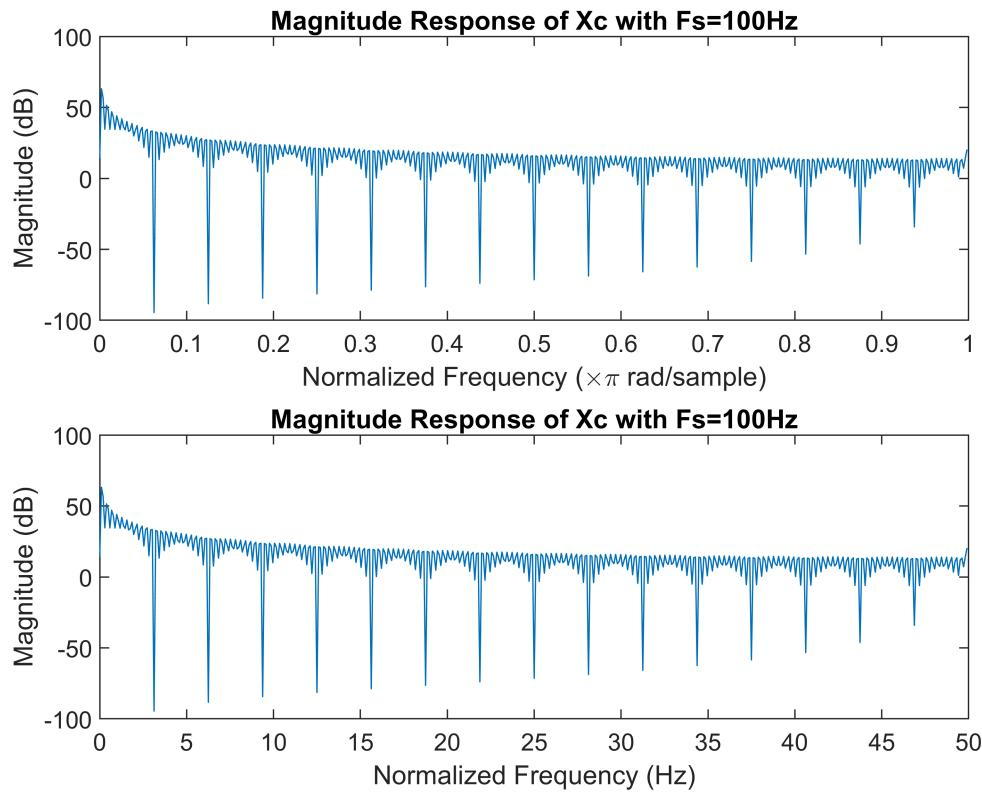
The original signal  $x_c(t)$  can't be recovered from  $x[n]$  because  $F_s = 100\text{Hz} < 2F_H = 2 \times (150)\text{Hz}$ .
