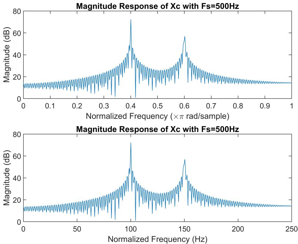
The original signal  $x_c(t)$  can be recovered from  $x[n]$  because  $F_s = 500\text{Hz} \geq 2F_H = 2 \times (150)\text{Hz}$ .
