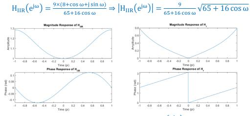
We can the curve of magnitude response of  $H_{IIR}(e^{j\omega})$  is smoother and larger than magnitude response of  $H_r(e^{j\omega})$ .
