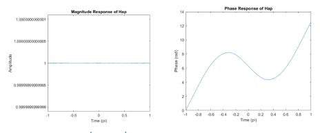
We can find that  $|H_{ap}(s)| = 1$  and  $\angle H_{ap}(s) + \angle H_{min}(s) = \angle H(s)$
