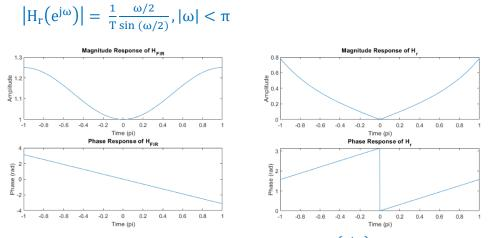
We can the curve of magnitude response of  $H_{FIR}(e^{j\omega})$  is smoother and larger than magnitude response of  $H_r(e^{j\omega})$ .
