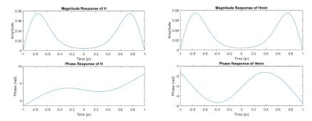
We can find that  $|H_{\min}(s)| = |H(s)|$  and  $\angle H_{\min}(s) < \angle H(s)$ (d) Briefly plot the magnitude and phase responses of  $H_{ap}(s)$ .
