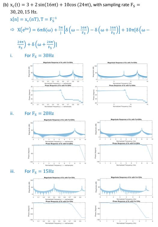
The sampling theorem shows that sampling signal can be recovered if  $F_S \ge 2 \times F_H$ , which  $F_H$  is 12Hz in the signal  $x_c(t)$ .
