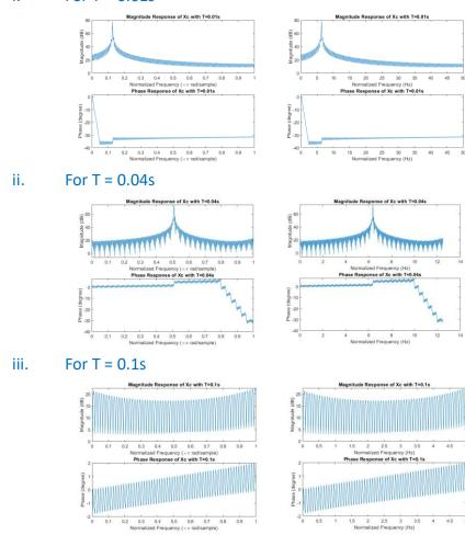
The sampling theorem shows that sampling signal can be recovered if  $T_H \ge 2 \times T$ , which  $T_H$  is  $\pi/35$  s, which equal to 0.089s, in the signal  $x_c(t)$ . Therefore, the sampling signals with T = 0.01s and 0.04s can be recovered.
