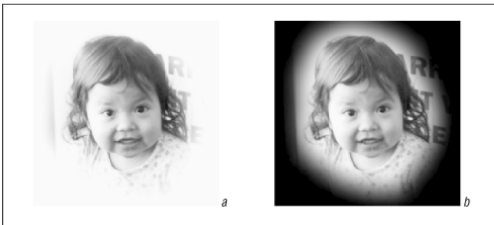
Figure 1-2: Portrait with an oval alpha mask (a) against a white background and (b) against a black background. (Click on images for full-scale versions.)
