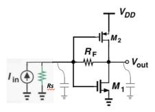
In this circuit, please use  $V_{DD}$ =1.5V. The shunt resistance  $R_F$  is assumed  $1K\Omega$  ohm. Input and output nodes are with 1pF load respectively. Current source is assumed with  $100K\Omega$   $R_S$  impedance.
