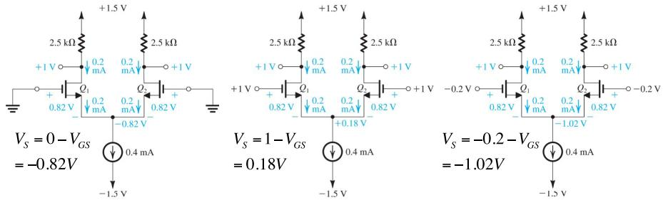
Maximum  $V_{CM}$  should keep  $Q_1$  and  $Q_2$  in Saturation
