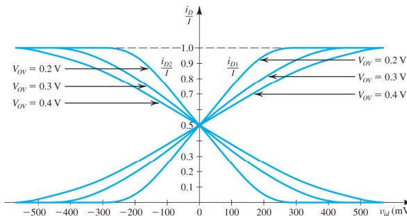
The linear range of operation of the MOS differential pair can be extended by operating the transistor at a higher value of  $V_{OV}$
