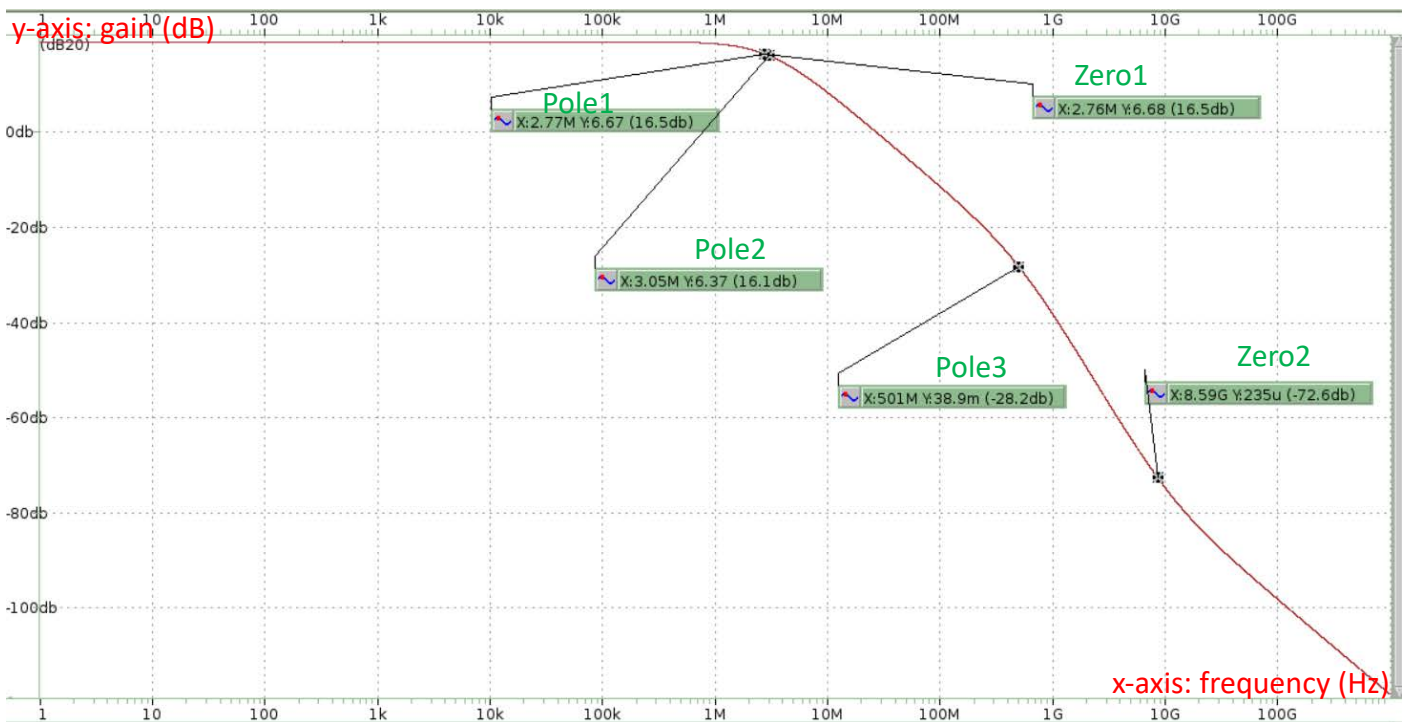
Fig. 6 Frequency response and poles & zeros analysis results
