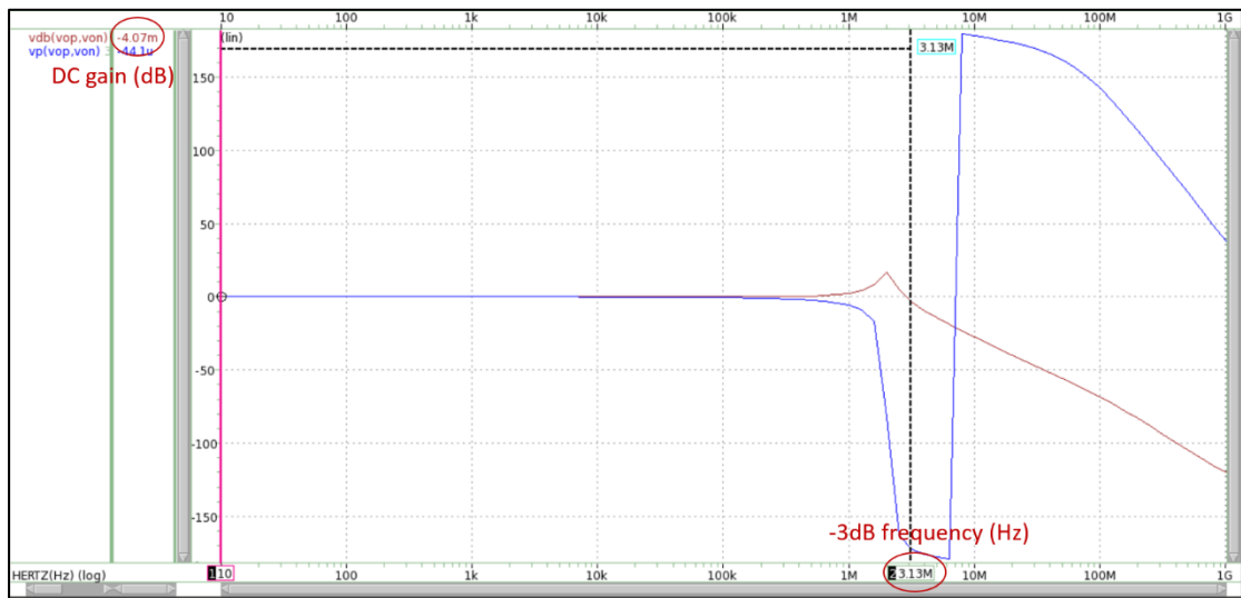
Fig. 3.7(b) AC magnitude and phase responses of differential mode gain
