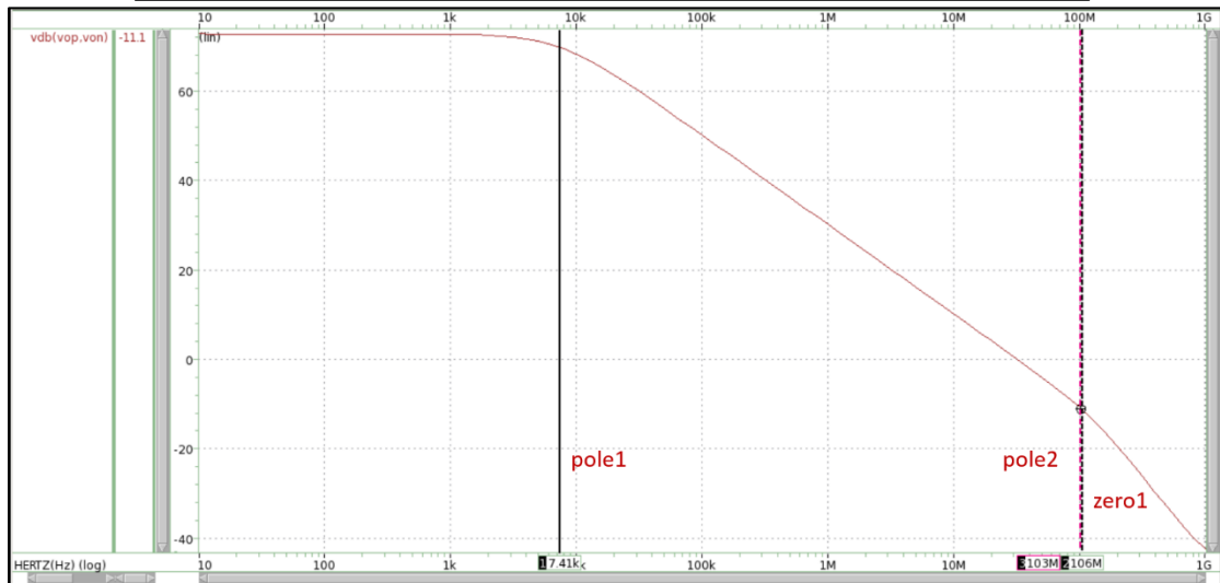
Fig. 3.1(c) Poles and zeros of differential mode
