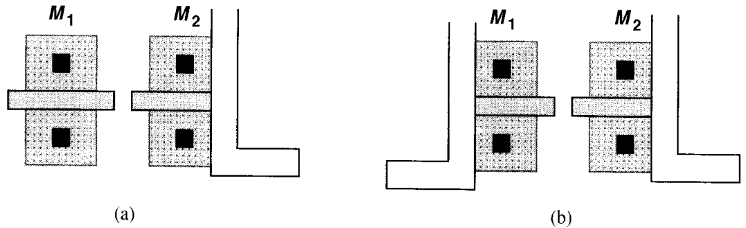
Figure 18.17 (a) Asymmetry resulting from a metal line passing over M_2 , (b) removing the asymmetry by replicating the line on top of M_1 .
