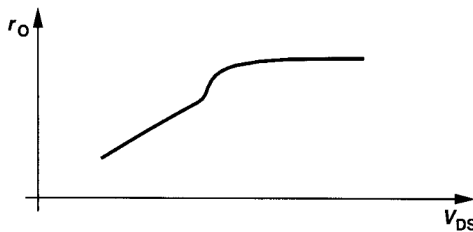
Figure 16.14 Kink in output resistance in Level 3 model.
