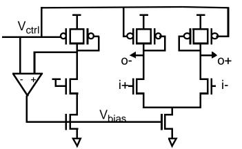
Replica loop keeps the swing of the buffers equal to Vctrl
