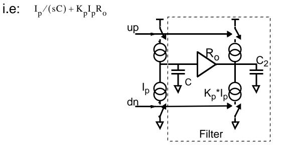
• If Ro and Ip are scaled appropriately, we can achieve scaling of the loop bandwidth with operating frequency [19]
