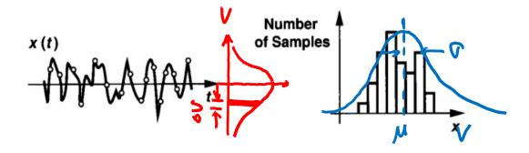
For example, a Gaussian distribution is defined by a mean and a standard deviation. We say the noise amplitude rarely exceeds  $4\sigma$ .
