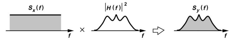
If a signal with spectrum  $S_X(f)$  is applied to a linear time-invariant system with transfer function H(s), the output spectrum is given by
