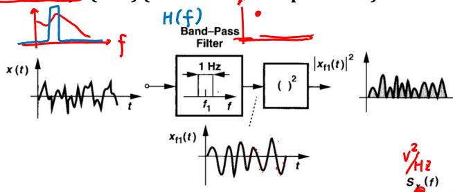
The PSD thus indicates how much power the signal carries in a small bandwidth around each frequency.
