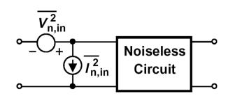
If the source impedance is high with respect to the input impedance of the circuit, then both must be considered.
