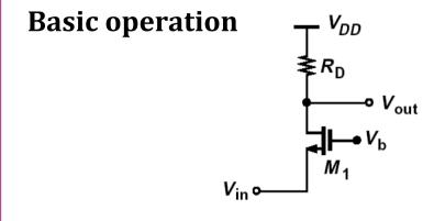
Due to the low input impedance, the input-referred noise current is not negligible even at low frequencies
