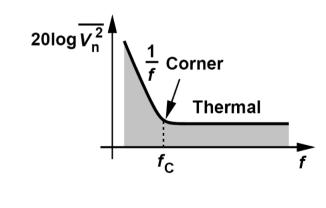
Where k is a constant and its value heavily depends on how 'clean' the process is. We often characterize the seriousness of 1/f noise by considering the 1/f 'corner' frequency.
