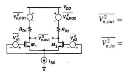
Thus, the input-referred noise voltage of a diff pair is 40% larger than that of a common-source stage – probably the only disadvantage of differential operation.
