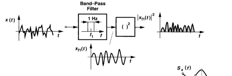
The PSD thus indicates how much power the signal carries in a small bandwidth around each frequency.
