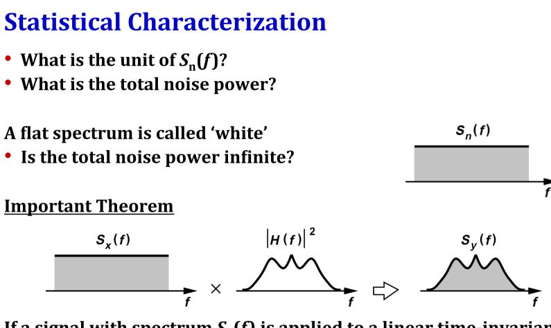
If a signal with spectrum  $S_X(f)$  is applied to a linear time-invariant system with transfer function H(s), the output spectrum is given by
