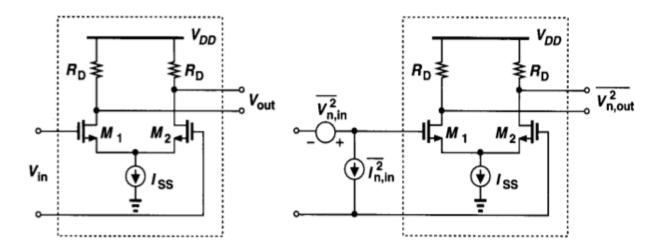
Since the four noise generators are uncorrelated, we can use superposition for the powers. Noise from  $M_1$ :
