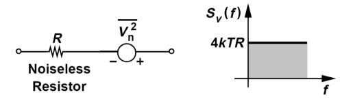
Note that the polarity of the voltage source is arbitrary.
