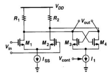
• As  $V_{\text{cont}}$  increases  $\rightarrow$  positive feedback
