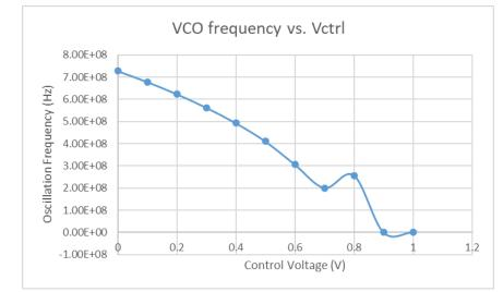
We can estimate the VCO gain at frequency 500 MHz is 0.37 V.
