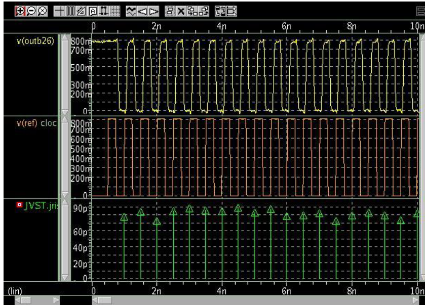
Figure 21 WaveView: Jitter vs. Time measurement to get Timing Interval Error (TIE) Jitter vs. Time. Measurement based on the reference signal
