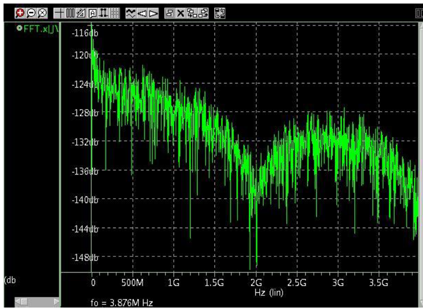
Figure 22 FFT of the TIE Jitter samples show the Jitter Spectrum
