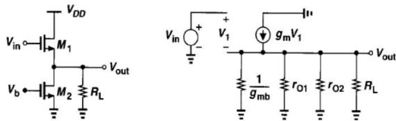
$$R_{out} = g_{m1} // g_{mb1} // r_{o1} // r_{o2} = 166.113 \Omega$$
