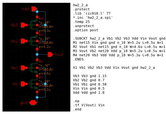
M1: W=5.2μm, L=0.5μm, Vin=0.5V M2: W=4.6μm, L=0.5μm, Vb1=0.58V M3: W=5.2μm, L=0.5μm, Vb2=0.7V M4: W=5.3μm, L=0.5μm, Vb3=1.15V
