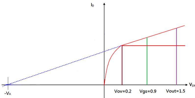
$$\begin{cases} I_{out} = K_n' \times 4 \times \left(\frac{W}{L}\right) \times (V_{GS} - V_{th})^2 \times \left(\frac{10 + 1.5}{10 + 0.2}\right), \\ I_{REF} = K_n' \times \left(\frac{W}{L}\right) \times (V_{GS} - V_{th})^2 \times \left(\frac{10 + 0.9}{10 + 0.2}\right) \end{cases}, I_{out} = 4 \times \left(\frac{10 + 1.5}{10 + 0.9}\right) \times I_{REF}$$
