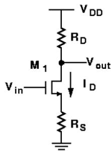
$$A_v = -G_m R_D = \frac{-g_m R_D}{1 + g_m R_s} = -\frac{R_D}{1/g_m + R_s}$$
