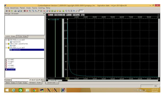
Therefore, based on the .lis file, the AC gain is about -149, and the output DC voltage is about 0.498 V with the input DC voltage designed with the value of about 0.387 V.
