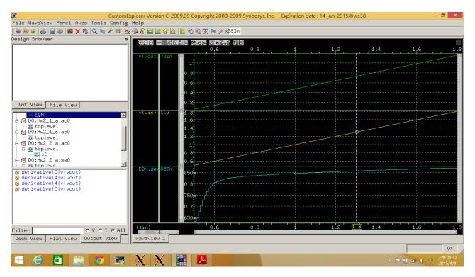
The source follower is designed with the bias voltage 0.45 V and the size W/ L = 5 u / 1.2 u and 5 u / 1 u for M1 and M2 respectively. At last, the gain becomes about 0.858.
