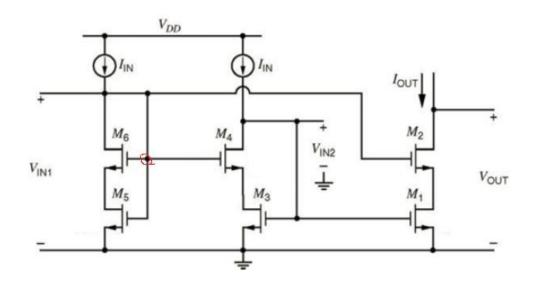
$V_{\rm in\,1}~$  = the voltage with red circle in the figure above =  $V_{\rm ov}~({\sf M3}) + (V_{\rm ov}~+~V_{\rm th}~)({\sf M4}) = 2V_{\rm ov} + V_{\rm th}$
