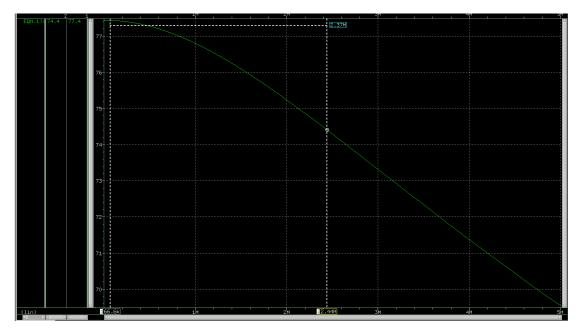
from the figure, -3dB bandwidth without  $C_p$  = 2.44M.
