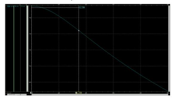
from the figure, -3dB bandwidth with  $\ C_p\$  = 1.73M.
