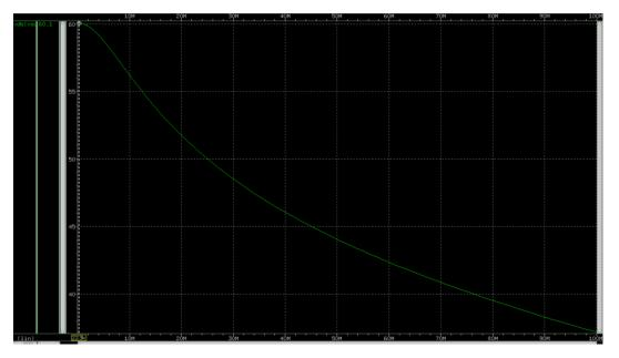
(b) Modify all the m(finger) in (a) to be double means to double the all the W in (a). And from the .lis file, we found it reasonable to have all the currents becomes two times of that of (a) since  $I_D$  is proportional to W, and all  $V_{dsat}$  remain the same, so  $V_{out-swing}$  is the same as (a).
