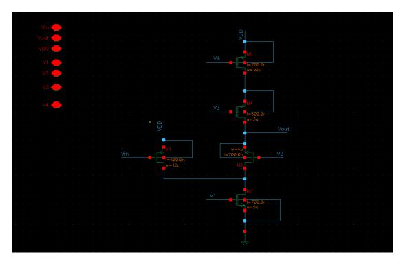
(a) My idea is: The ac gain is proportional to  $g_{m1}$ , so if we want a bigger gain, I design  $g_{m1}$  to be bigger. And design to make  $I_{d3} = I_{d4} = I_{d5} + I_{d1}$  as close as possible to 40uA, and meanwhile, keep all mos in saturation.
