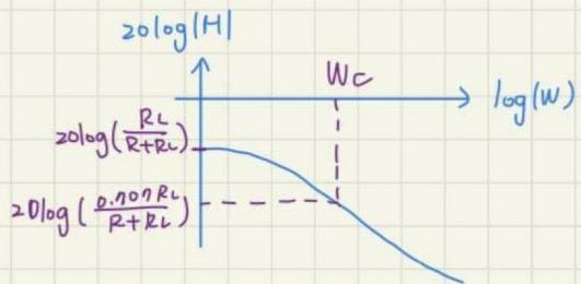
$$\text{when } w_c = \frac{1}{C \cdot \frac{R \cdot R_L}{R+R_L}} = \frac{R+R_L}{R \cdot R_L \cdot C}$$
