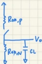
$V_{o, initial} = V_s, V_{o, final} = 0$
