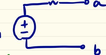
1)  $V_{TH}$ :  $\left\{ \begin{array}{l} KCL @ a: \frac{V_a - 24}{2} + 4 + 3i_x + i_x = 0 \\ \Rightarrow V_a = 8V = V_{TH} \end{array} \right.$
