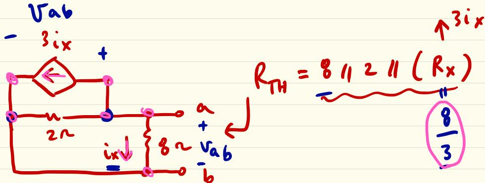
$$= \frac{1}{\frac{1}{8} + \frac{3}{8}} \parallel 2 = 2 \parallel 2 = \underline{1\Omega}$$
