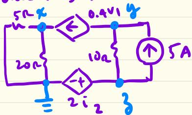
$$\text{KCL at } X: \frac{V_x}{5} + \frac{V_x}{20} - 0.4V_1 = 0$$
