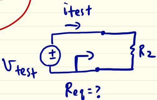
$$\frac{V_{test}}{i_{test}} = R_2$$
