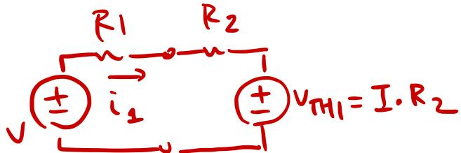
$$i_1 = \frac{V - V_{TH1}}{R_1 + R_2}$$
