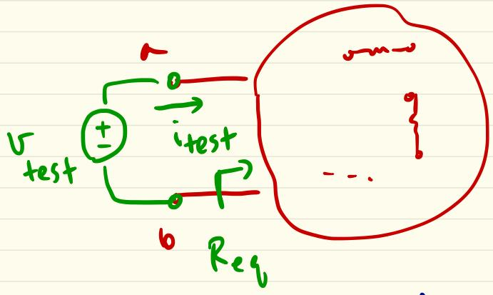
$$Req = \frac{V_{test}}{i_{test}}$$
