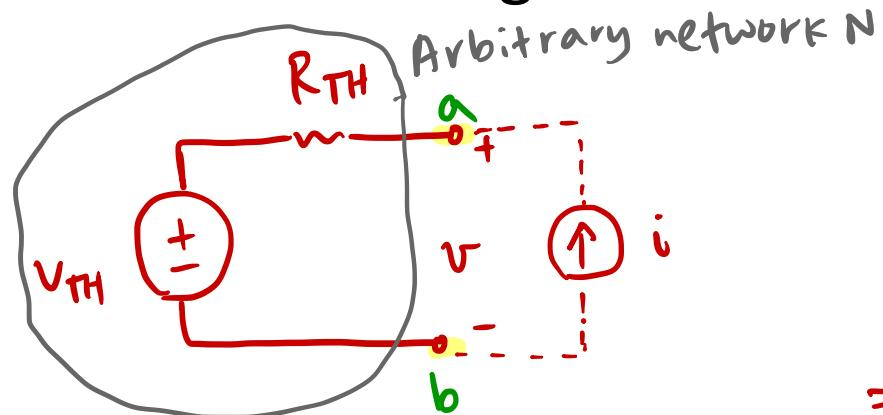
$$v_{TH} = v_{open} \Big|_{i=0}$$
