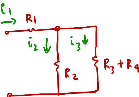
$$Req_1 = \frac{R_2(R_3+R_4)}{R_2+R_3+R_4}$$
