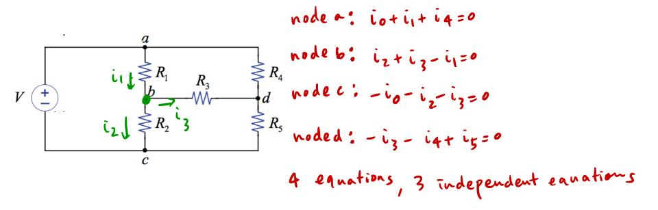
Basic KVL/KCL Method of Circuit Analysis
