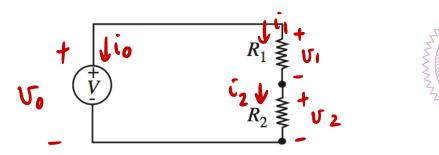
An isolated loop with >2 resistors and a voltage source in series.
