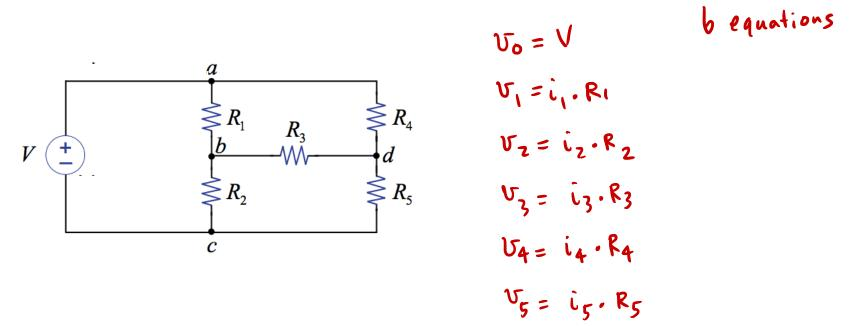
Basic KVL/KCL Method of Circuit Analysis
