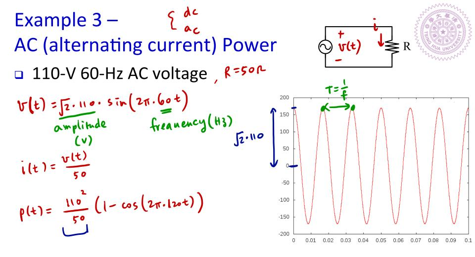
What would be the power dissipated by the resistor if the voltage was a constant value of 110 V?
