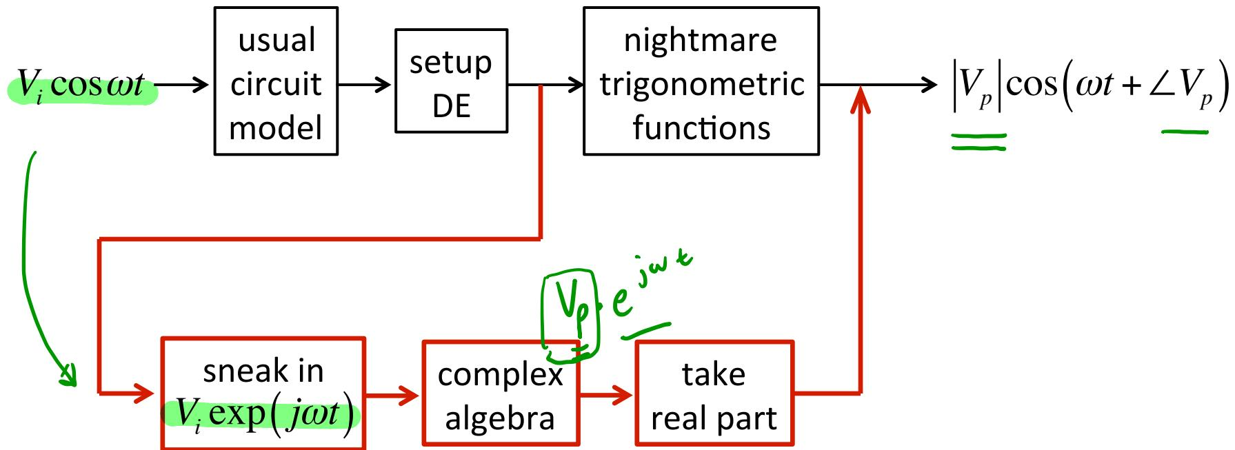
$$V_p = \frac{V_i}{1+j\omega RC} \quad \text{complex amplitude}$$
