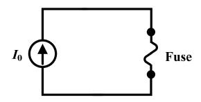
Use the following data to determine the current  $I_{max}$  at which the fuse will blow (i.e., its temperature goes up without limit). (10%)
