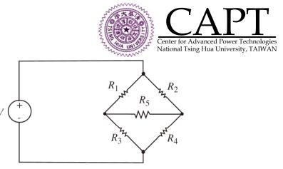
Replacing network N with its Thévenin equivalent
