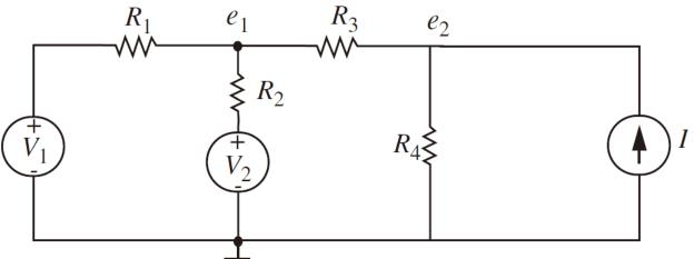
• Set  $V_2$  and I to zero to find the voltage component  $e_{IA}$  of  $e_1$  due to source  $V_1$  acting alone.
