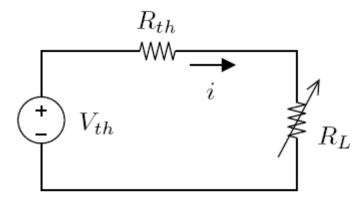
$$i = \frac{V_{TH}}{R_{TH} + R_L} \rightarrow P_L = (\frac{V_{TH}}{R_{TH} + R_L})^2 R_L$$
