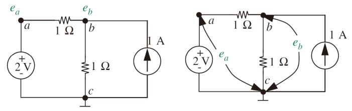
Although the choice of *reference node* is in fact arbitrary, it is most convenient to *choose the node that has the maximum number of circuit elements connected to it*. The potential at this node is defined to be zero V, or ground-zero potential.
