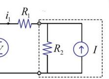
Replacing network N with its Thévenin equivalent
