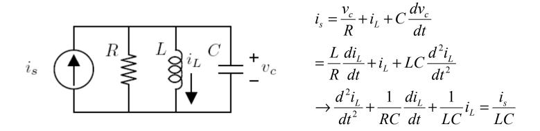
• For  $\underline{i_s} = 0$ , the <u>natural response</u> of the circuit can be derived:
