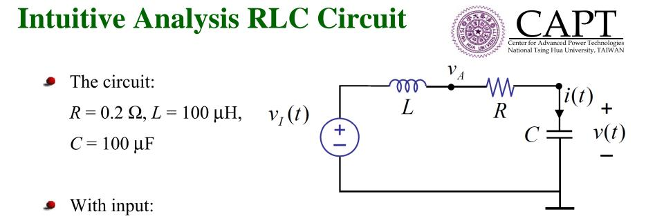
$v_I(t) = V_I u(t)$  where  $V_I = 1$  V
