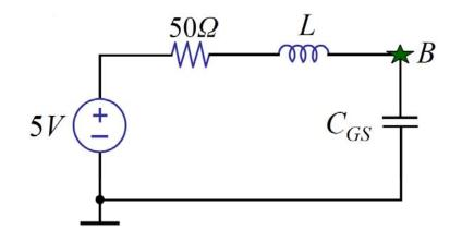
Under smaller R of 50  $\Omega$ , the series RLC circuit become *underdamped* and the *ringing* occurs.
