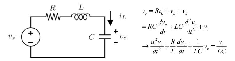
• For  $v_s = 0$ , the <u>natural response</u> of the circuit can be derived:
