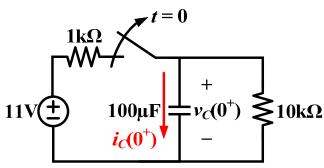
Since the voltage across the capacitor must be the same as the switch is opened, i.e.  $v_C(0^+) = v_C(0^-)$ , thus  $v_C(0^+)$  and  $i_C(0^+)$  can be found from the above two circuits.
