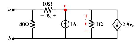
The open circuit voltage at port ab is the Thévenin equivalent voltage  $v_{TH}$ .
