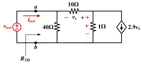
$$R_{TH} = \frac{v_{test}}{i_{test}} = \frac{v - v_x}{\frac{v_{test}}{40} - \frac{v_x}{10}} = \frac{\frac{-40v_x}{10}}{\frac{-v_x}{10} - \frac{v_x}{10}} = \frac{40}{2} = 20\Omega$$
