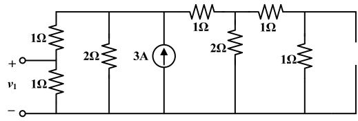
The  $v_{3A}$  can be found as  $v_{3A} = 3 \times \frac{2}{1+2} \times \frac{1}{2} \times 1 = 1V$
