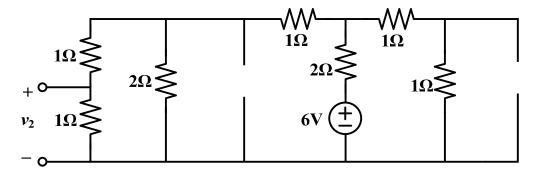
The  $v_{6V}$  can be found as  $v_{6V} = 6 \times \frac{1}{1+2} \times \frac{1}{2} \times \frac{1}{2} \times 1 = \frac{1}{2} V$
