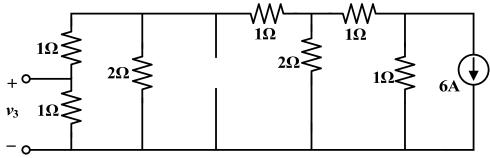
The  $v_{6A}$  can be found as  $v_{6A} = (-6) \times \frac{1}{1+2} \times \frac{1}{2} \times \frac{1}{2} \times 1 = \left(-\frac{1}{2}\right) V$
