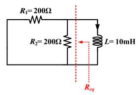
$$\Rightarrow \tau = \frac{L}{R_{eq} = (R_1 || R_2)} = \frac{10m}{100} = 10^{-4} (\text{sec})$$
