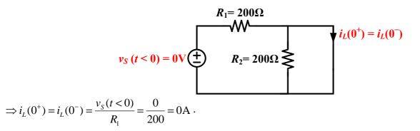
2. To find the final value (at  $t = \infty$ ), the inductor should be regarded as a short circuit with a stable 10V voltage input signal.
