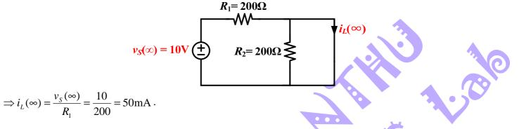
3. Before determining the time constant, we need to set the independent source to zero, and find the equivalent resistance  $(R_{eq})$  connected with the inductor's terminal.
