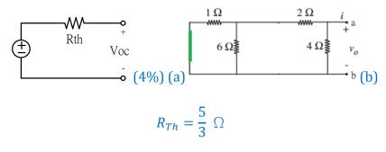
For finding Voc, we use superposition method. Turn off the current source.
