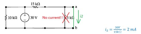
Turn off the 10mA current source and 30V voltage source.
