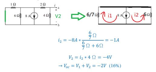
6. Find the Norton equivalent of the circuit at terminal ab in the following figure. (20%)
