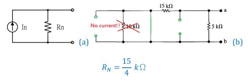
For finding In, we use superposition method. Turn off the 30V voltage source and 3mA current source.
