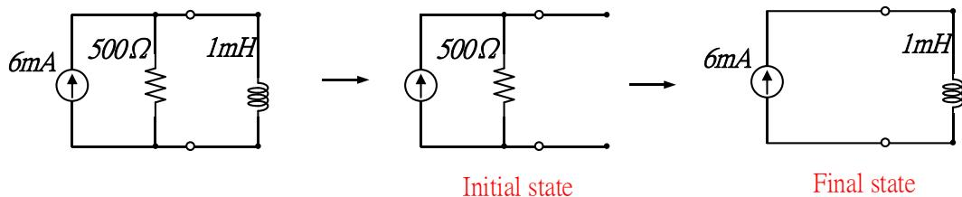
For  $t > 0$ , the inductor just like open circuit at initial state
