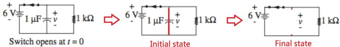
For  $t > 0$ , the capacitor just like short circuit at initial state
