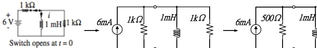
For an easy way to calculate, we may transfer the circuit into Norton equivalent.
