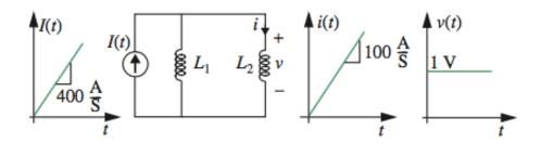
4. A constant current source having value I drives a time-varying inductor shown in the following figure. The inductance is  $L(t) = L_0 + L_1*\sin(\omega t)$ . Determine the inductor voltage v(t).
