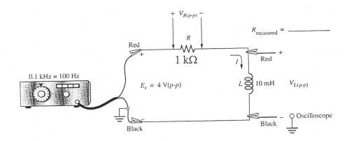
(3) (5%) For the circuit below, the input ac voltage magnitude  $E_{p-p}$  is related to the magnitudes of  $V_{R(p-p)}$ ,  $V_{c(p-p)}$  and  $V_{L(p-p)}$ . Please <u>analyze</u> and give the expression of  $E_{p-p}$  in terms of  $V_{R(p-p)}$ ,  $V_{c(p-p)}$  and  $V_{L(p-p)}$ . 不需將電壓、電阻、電容及電感的值代入來計算實際值.
