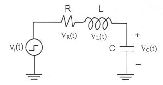
(2) (8%) For the same circuit (but the input is now a <u>sinusoidal waveform</u> from low to high frequencies), please <u>analyze</u> and roughly sketch the frequency responses of  $V_R$ ,  $V_L$ , and  $V_C$  (magnitude vs. frequency only). Please mark the natural frequency of the circuit and indicate whether the maximum values appear before or after the natural frequency. (Hint: 不需將電壓、電阻、電容及電感的實際值代入作計算)
