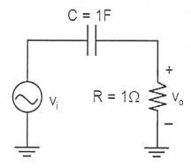
(4) (4%) For the R-C circuit above, the input  $v_i(t)$  is a unit-step and the initial voltage on the capacitor is zero, please calculate the output voltage  $v_o(t)$ .
