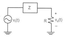
(2) (8%) Find the transfer function  $v_2(s)/v_i(s)$  of the filter as shown.
