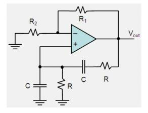
(b) (10%) For the triangular, square-wave oscillator as show:  $R_1 = 4R_2$ ,  $R = 1 \text{ k}\Omega$ ,  $C = 0.1 \mu\text{F}$ , and the output  $V_o$  oscillates between ±10 V. Please point out where the triangular wave and square wave are produced, respectively (namely, point A or point B). Also, please calculate the oscillation frequency of the circuit.
