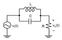
$$\frac{v_{o}(s)}{v_{i}(s)} = \frac{s^{2} + \frac{1}{LC}}{s^{2} + \frac{1}{RC}s + \frac{1}{LC}}$$
