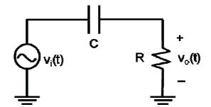
$$\frac{v_{o}(s)}{v_{i}(s)} = \frac{R}{R + \frac{1}{sC}} = \frac{sRC}{sRC + 1}$$
