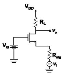
Compared to the common-source amplifier, CG's overall voltage gain is smaller by a factor of about  $1+g_m R_{sig}$ .
