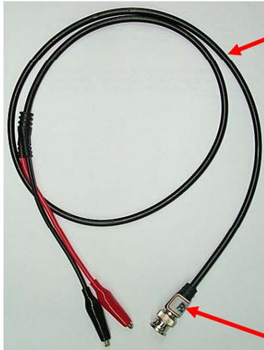
**Coaxial cable:** a type of wire that consists of a center wire surrounded by insulation and a grounded shield of braided wire. The shield minimizes electrical and radio-frequency interferences
