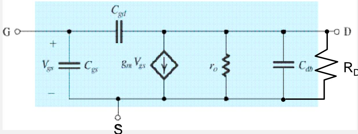
Note: Make sure that  $V_{ds} > V_{gs} - V_t$  for the transistor to operate in the saturation region
