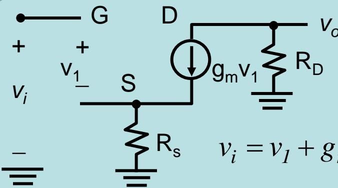
$$v_i = v_1 + g_m v_1 R_s \Rightarrow v_1 = \frac{v_i}{1 + g_m R_s}$$
