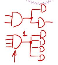
The decoder size and the number of inputs per gate can be reduced by using a coincident selection in a 2D array.
