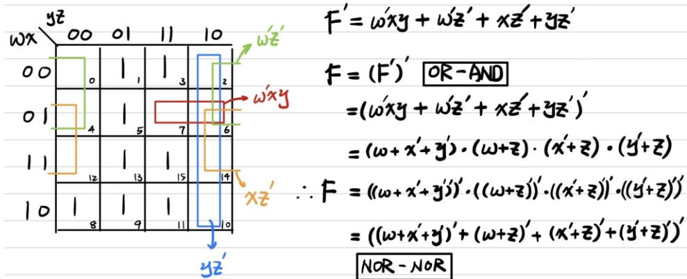
6. (20%) Simplify the following Boolean function F, using the two-level forms (a) AND-OR-Inverter, (b) OR-AND-Inverter logic diagrams
