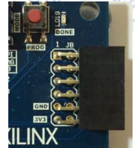
Figure 20. Pmod connectors; front view as loaded on PCB.
