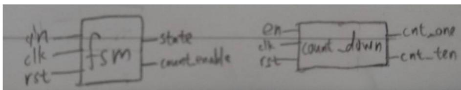
**1.3 Use a FSM to implement the function of pause/start function. Use one LED to represent current state.**
