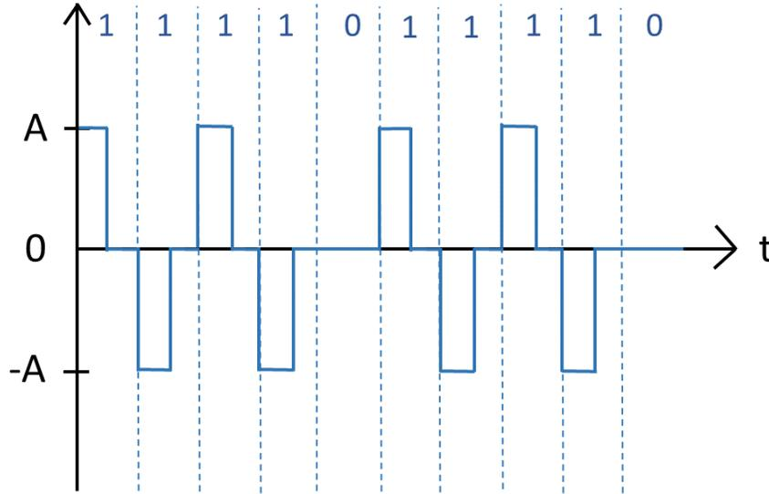
Figure 4: Bipolar return-to-zero signaling in Problem 5.(a).
