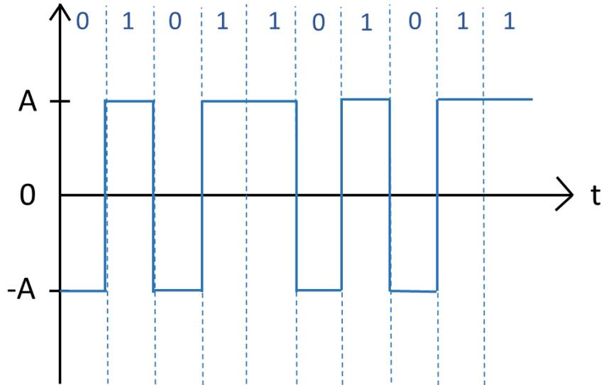
Figure 5: Polar nonreturn-to-zero signaling in Problem 5.(b).
