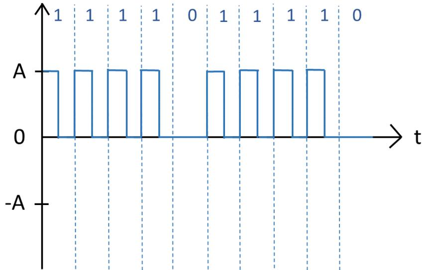
Figure 3: Unipolar return-to-zero signaling in Problem 5.(a).
