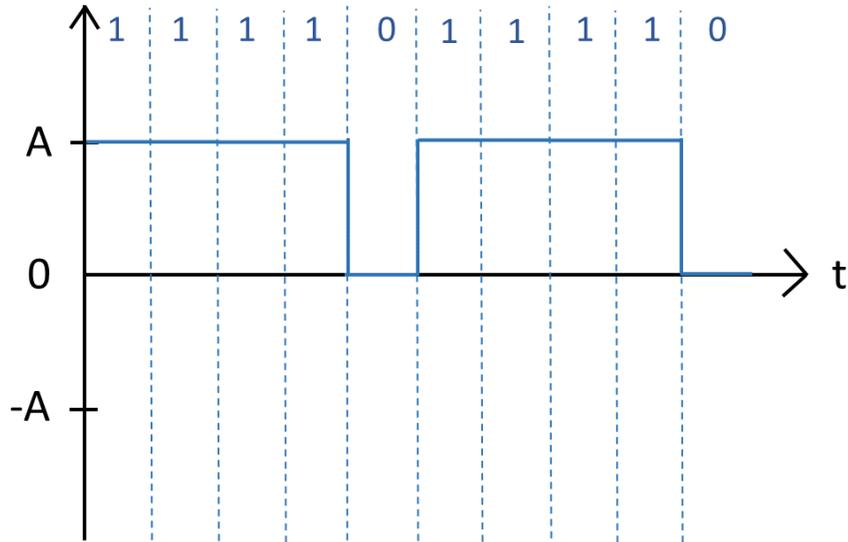
Figure 2: Unipolar nonreturn-to-zero signaling in Problem 5.(a).
