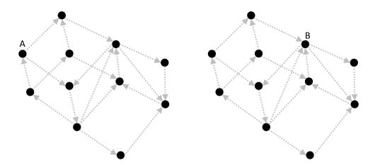
2. How many **independent cycles** are there in the following circuit? Hint: view the circuit as a graph.
