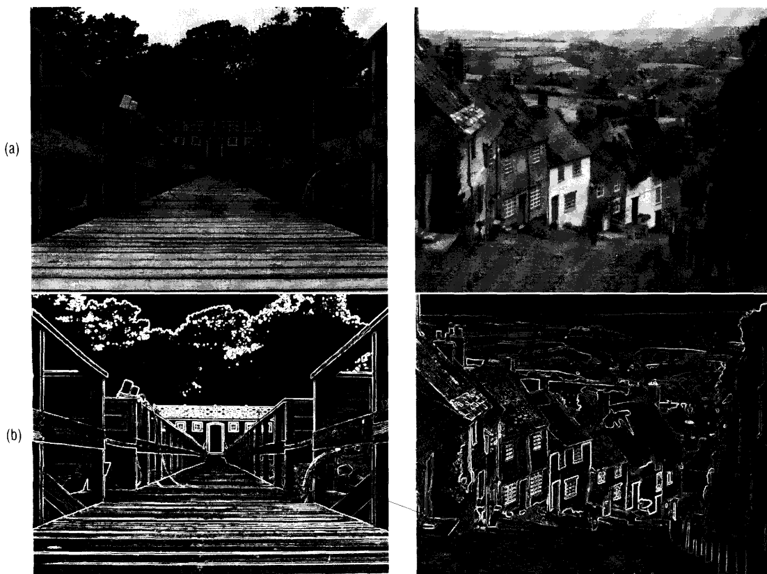
Figure 3.24 Effect of a differentiating filter on an image: (a) two original images; (b) the result of processing the original images with a differentiating filter.
